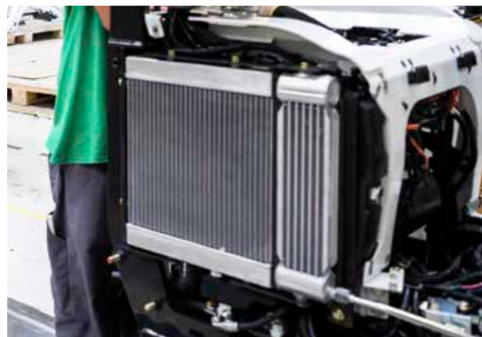
Hydraulic oil cooler
